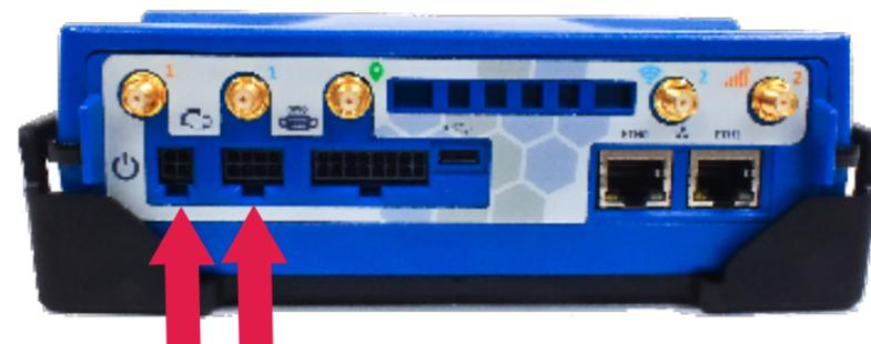
**3** Connect the power cable to turn on the modem.
