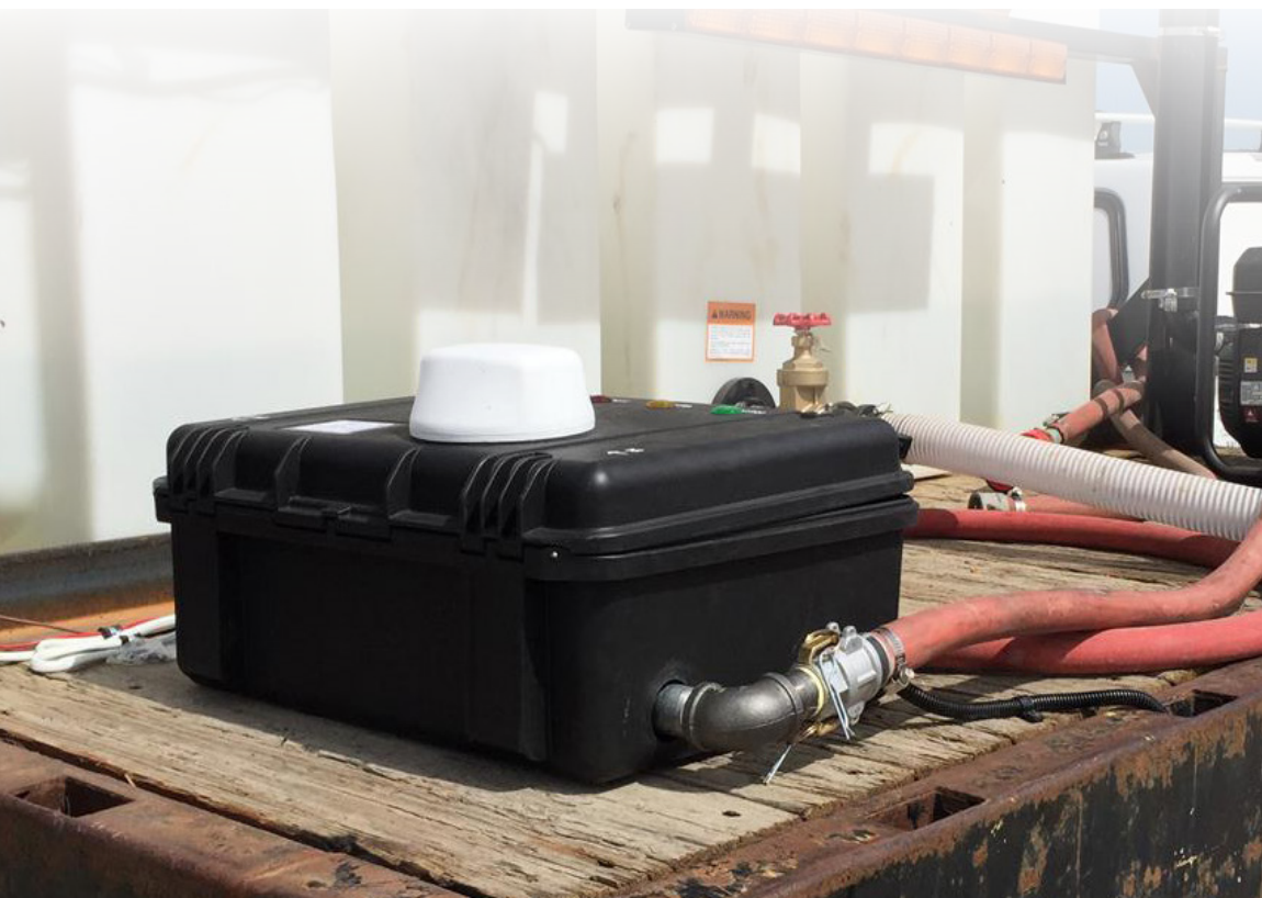
Image 2: Flow control system installed on a tree watering truck
