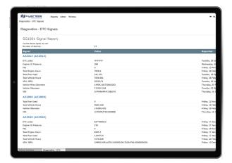
When your CTM hardware is connected to the vehicle CAN Bus, the CTM will detect the malfunction indicator light (MIL) status and the number and type of trouble codes. Set up real-time alerts in Cypress VUE when a MIL light is activated along with the associated trouble codes. Monitor fleet maintenance needs in no time.
