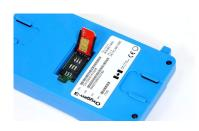
Ensure the contact area of the SIM card is visible and that the chamfer corner (angled corner) of the SIM card is located as shown.
