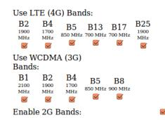
Depending on the cellular module installed in the Oxygen-3 modem, there may be more or less bands that can be selected – the module used in the example above is the MC7354.
