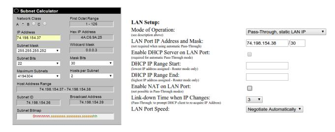
In the above example, the Oxygen-3 Wireless Gateway's LAN port is configured as 74.198.154.38/30, while the connected device is configured with the real wireless carrier IP of 74.198.154.37/30.
