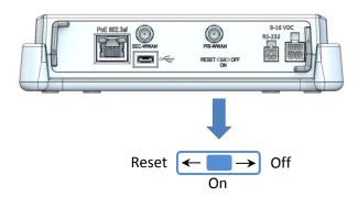
The Oxygen-3 Wireless Gateway has a small 3-way switch on the back panel which serves as a power and reset switch.
