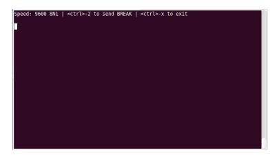
Press <ctrl> - 2 to send a break signal (for example to enter ROMMON mode on a Cisco® router) Press <ctrl> - x to exit from the terminal software
